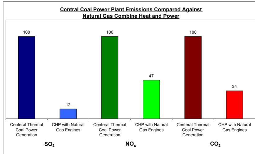
Figure 3: Comparison of emissions from central coal power production to natural gas combined heat and power for the same quantity of power produced. <sup>1</sup>
