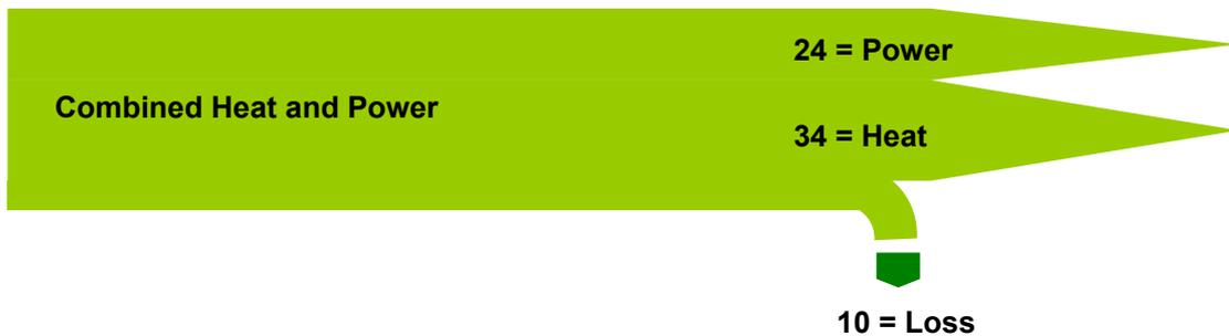
*Figure 5: Energy flow diagram comparing separate heat and power plants versus 1 combine heat and power plant to accomplish both. It is evident that using combined heat and power saves 30% of the energy regardless of the energy source.<sup>1</sup>*
